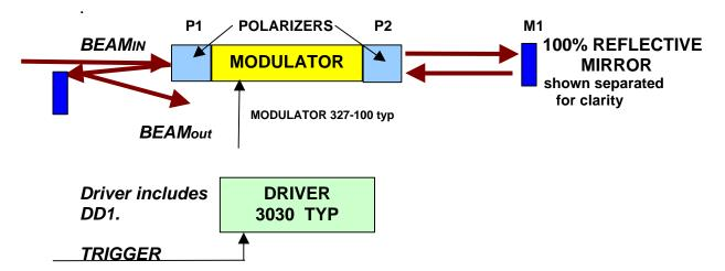
The input beam is vertically polarized and transmits through the vertically oriented input polarizer. When a voltage is applied to extinguish the beam, a small residual component passes through the output crossed polarizer and retro-reflects back through the input optics. Since this component is horizontally polarized, it is rejected by the input polarizer almost completely. The degree of extinction is dependant on the angular deviation between the input beam and the useable reflected beam.
